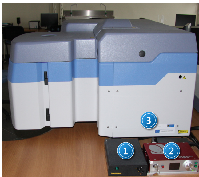
Picture 2. Measurement apparatus – side view: 1 – He-Ne laser power supply; 2 – YAG:Nd laser power supply; 3 – Raman spectrometer.
